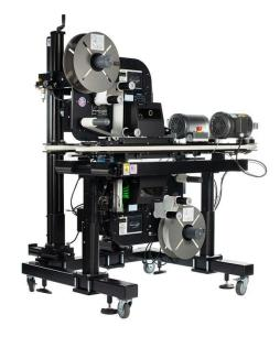
The final Panther Industries labeling automation solution for Mountain Man Nut & Fruit Co., incorporating two Panther P8 pneumatic label applicator systems integrated with a hugger belt and corresponding outriggers.
