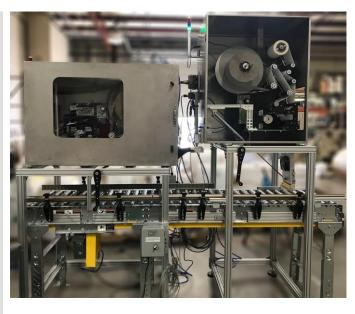
FOX IV designed a two unit, integrated labeling station to label the various feed block products.
