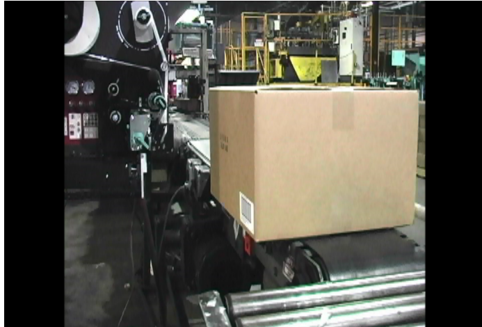
A FOX IV Intermec-based Print and Apply system places the bar code label on the side of each case of glassware.
