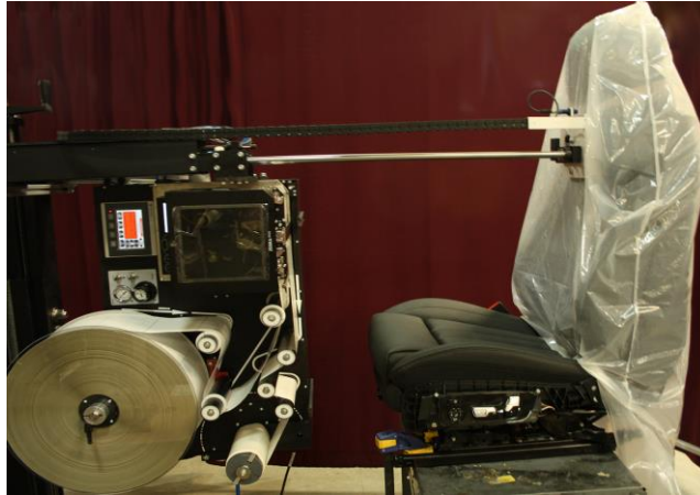
FOX IV's 6956 Zebra based print and apply labeling system applying a 6" x 4" label to the plastic cover of automotive front seats.
