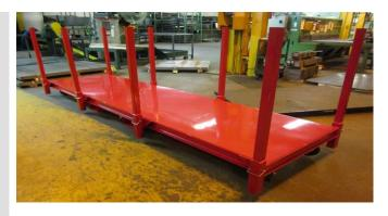
An international manufacturer of pressure rated plastic pipe and valves approached Abel Womack International Handling of Lawrence MA with a set of problems. The existing stacking carts that hold the pipe prior to processing were a safety concern. The carts were being stacked 4-5 high, putting excessive strain on the bottom cart. Also accessibility to the lower carts was prohibited until the top carts were moved via lift truck. Safety and efficiency were the concerns.
