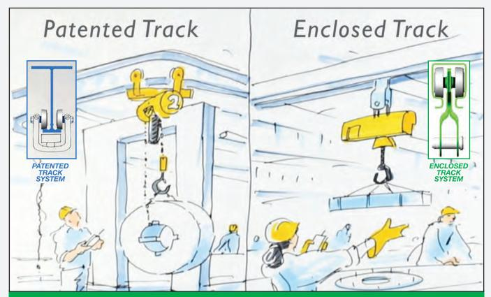
For effectively transporting loads up to 40 tons in a productive and safe manner, patented track systems feature an inverted "T" design with a machined running surface that ensures smooth trolley travel with little wear. The hard alloy steel profile provides long life even in heavy duty applications. The articulating design of the trolley provides equal wheel loading, leading to extended life of patented track systems, even in severe environments.
