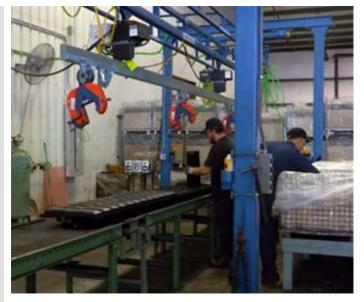
A manufacturer of track for large, earth moving equipment, (Bulldozers etc...), needed to design a new work cell that would allow workers to safely flip the track during production.
