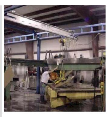
This customer fabricates countertops using granite and marble. In this application, workers at a new facility need to move huge slabs of granite from station to station through the various stages of the fabrication process.
