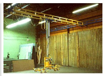
A glass mirror manufacturer makes large mirrors for the furniture industry. In the packaging process of these mirrors, the large, heavy (up to 300 lbs.) sheets of glass must be lifted off a conveyor, tilted 90 degrees, and then placed in a wooden shipping crate. To keep the fabrication process running efficiently, one mirror must be lifted and placed in the crate every 60 seconds.
