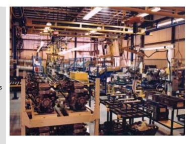
An automotive manufacturer in Canada needed a process for overhead material handling when their plant converted from a warehouse operation to a manufacturing operation. They chose Free Standing Bridge Crane systems to serve their engine/transmission assembly lines because the building could not support Ceiling Mounted Bridge Cranes. The bridge crane system has three bridges on a single runway which is 86' long. Each bridge serves a work area that is approximately 28' long.
