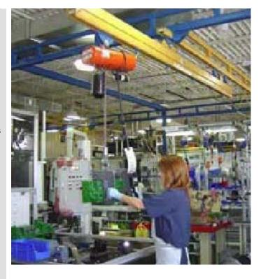
Gorbel's Work Station Crane with telescoping bridges provided a Wisconsin valve maker with a cost effective way to handle a growing work cell.
