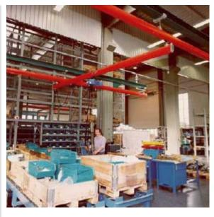
The force required to begin movement is approximately 1% of the load being moved.
