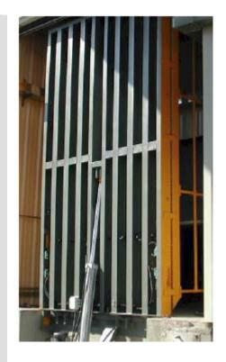
A bascule bridge permits safe crossing of railroad spurs and serves as a convenient connection between buildings. This is exactly what a distributor of pet care products needed to bridge the gap between their main warehouse and the outdoor staging area, while still allowing the frequent railcar to travel between the two buildings. The bascule bridge was the answer to safe and productive material movement throughout the facility.
