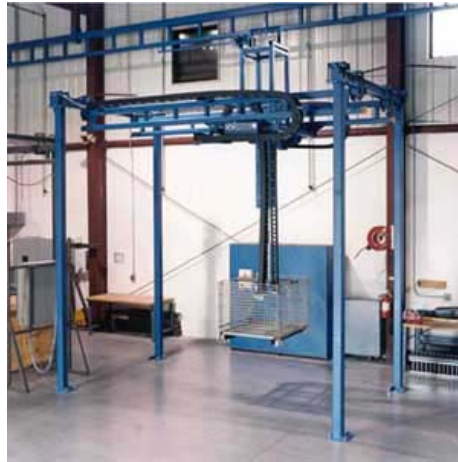
Figure 4. Workstation crane for a work cell.
