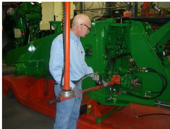
Figure 5 Manipulator in Assembly Operation at Large Vehicle Manufacturer. Operator can safely and effectively position an awkward 40 lb part. Previously the operator was forced to lie on the floor in a supine posture to position and affix this part.
