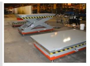
Load cell lift system for weighing pipes eliminate risks of overloading crane.
