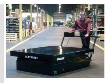
Custom built Series 35 EXW Scissors Lift Cart built with wheeled transport base and battery operation allows for easy maneuvering to various work stations within plant environment.
