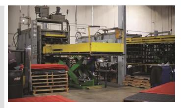
8,000 lb. capacity Kelley lift tables raise trays at M+A Matting to the appropriate height for rubber material to enter ovens for curing prior to further commercial floor mat production.
