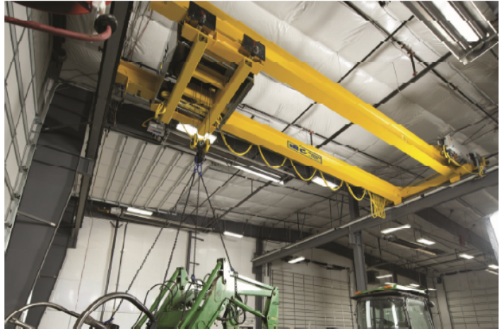
Ultra-compact double girder under-running hoist design
