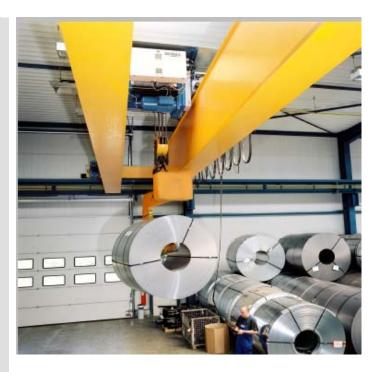
Handling steel coils is challenging when the operator would like high lifting speeds combined with safe load spotting. This coil processor needed both: heavy duty design and "smooth" high speed lifting. The Demag DR Pro Hoist provides the needed ruggedness and sensitive speed control from a standardized hoist to meet the duty requirements of steel coil handling and processing.
