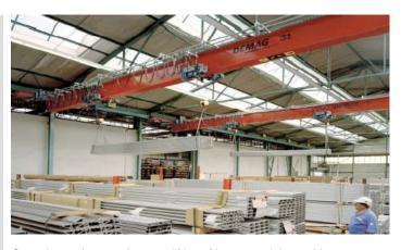
Smooth, precise, synchronous lifting of long materials provides an efficient and safe operation.
