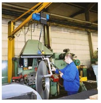
A Demag DCS Electric Chain Hoist was selected for this application due to its stepless variable speed lifting capability. The operator can easily control the lifting and lowering speed of the hoist over a wide range from 0.5 - 50 feet per minute or any speed in between.
