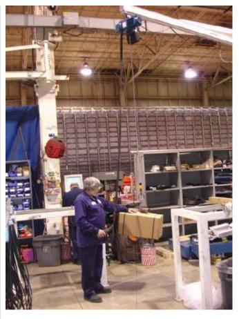
A Demag Electric Chain Hoist combined with an Enclosed Track Jib Crane provide an excellent material handling solution.
