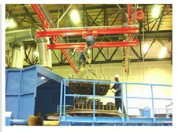
A manufacturer of Plastic components needed a precise and reliable solution for the handling of special heavy molds. The solution was to use 2 each 4000lb capacity Demag Electric Chain Hoists suspended from a KBK3 Enclosed Track System.
