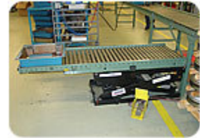
A transmission manufacturer uses a scissor lift attached to a roller conveyor on its assembly line.
