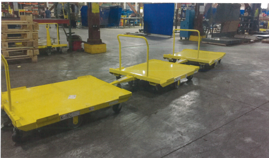
A train of flat deck carts is used to move materials around the facility and to the production lines. Photos provided by K-Tec Inc.
