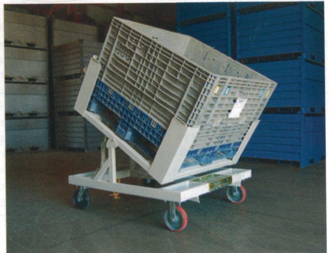
A tilt cart. Photo provided by Topper.
