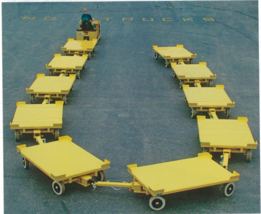
A train of Quad steer carts pulled by a tugger. Photo provided by Topper.
