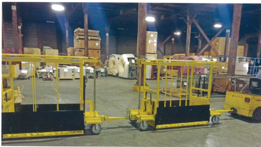
A train of mother carts with ramps on either side that allows for the loading/unloading of existing daughter carts to be moved to production lines. Photos provided by K-Tec Inc.
