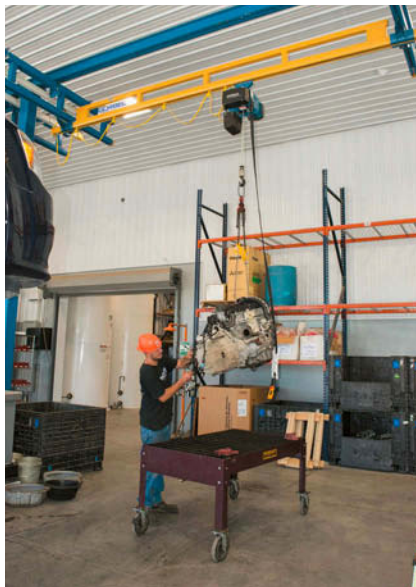
The five-bay freestanding workstation crane at Wilbert's Automotive Recycling in Webster, NY, pulls engines from automobiles so they can be put into inventory for sale. One bay has a dual bridge; one lifts the cab of a pickup truck while the other pulls the engine. Photo courtesy of Gorbel.
