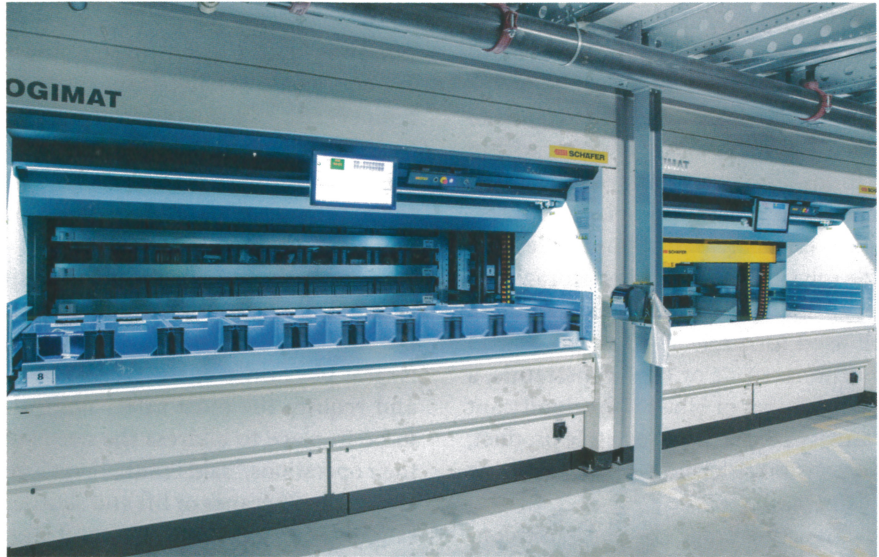
The SSI SCHAEFER LOGIMAT Vertical Lift Module
