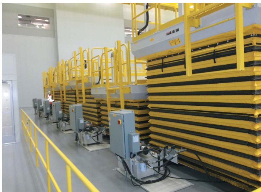
These six partially raised hydraulic work access lifts raise, lower and position workers to gain good ergonomic access to their work. The work area is behind a barrier and the lifts are fitted with handrails with spill guards, gates and ladders for egress on and off the platforms.
