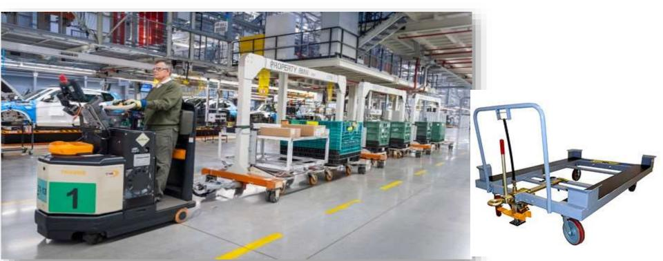
Look to positioning devices when the towable cart is placed in the work cell
