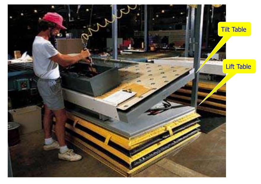
The challenge is simply giving the assembler total access to work lift and tilt devices provide ready that access
