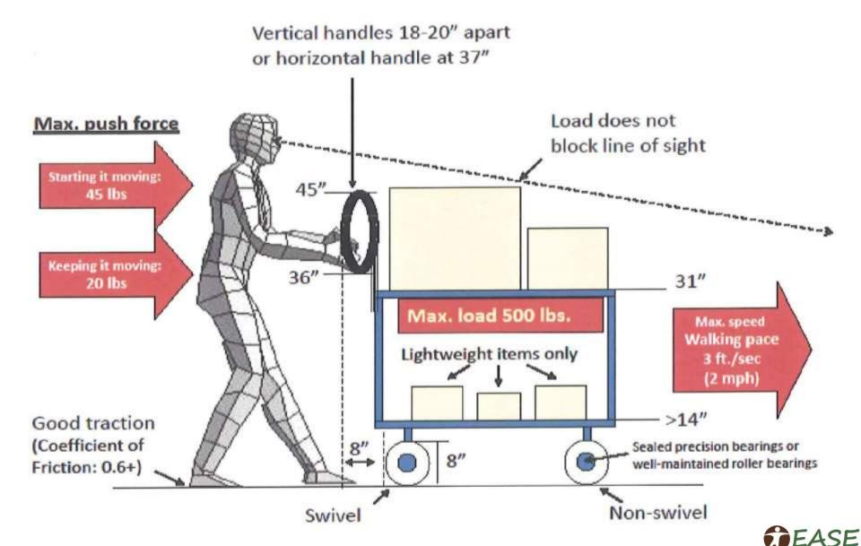
The wheel choice can have a huge impact on the rolling friction of any cart, dolly or portable rack.
