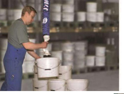
Vacuum tube lifters are highly efficient for handling cartons, bags and pails
