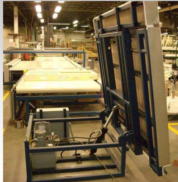
Hydraulic tilt table for large window assembly
