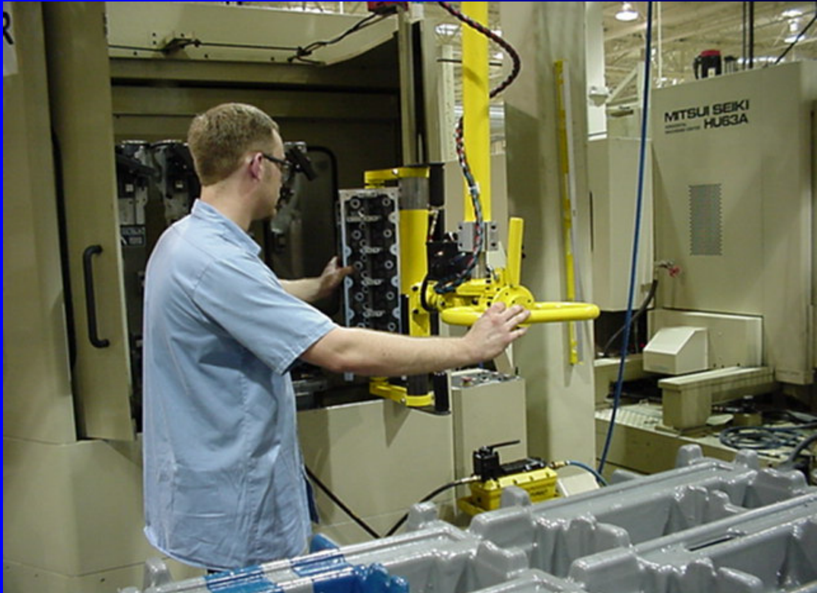
Manipulators making easy work of handling cylinder heads in a machining center
