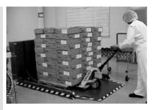
A manufacturer of prescription drugs, recently added state- of-the-art work positioning tables to prevent back strain for its employees working on production lines. Since the addition of seven customized roll on Level Loaders there has been a lot less bending and lifting at the plant.
