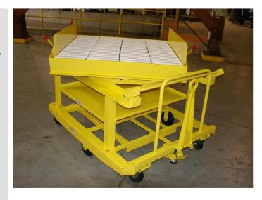
Rotate conveyor cart compatible for tugging in a train or manual pushing and pulling.
