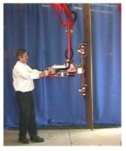
The box is picked up off the pallet with a custom designed vacuum tool. The box is pitched 90 degrees to a vertical postion.
