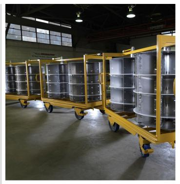
Three of the 68 carts designed specifically for delivery of parts to the assembly line in a lean manufacturing facility.
