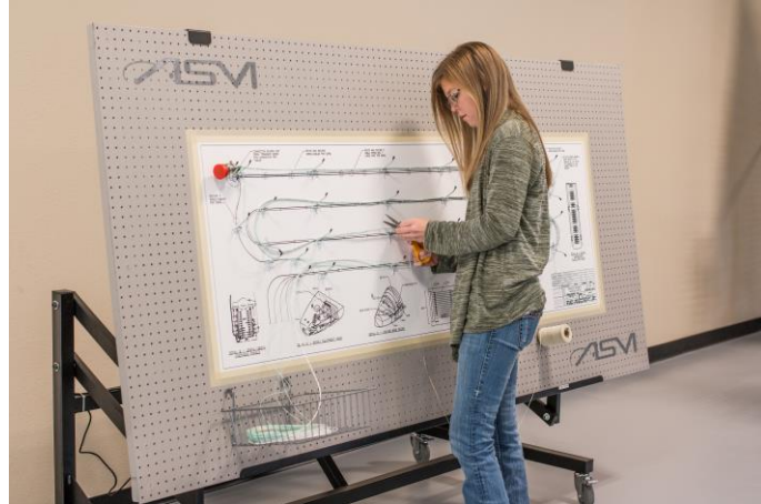
Aircraft Systems and Manufacturing (ASM) processor utilizing a BOSTONtec wire harness board workstation.
