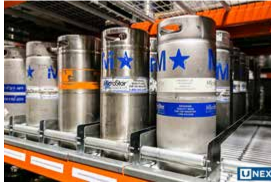
Sixtel kegs are stored in Span-Track carton flow positions at Atlas’ distribution center
