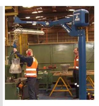
Nissan Castings is an Australian castings plant for transmission housings. In this work cell, they were loading and unloading alloy transmission castings into a jig where a quick machining process takes place.
