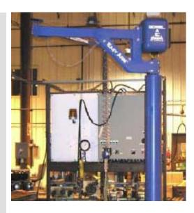
The first work cell (see work cell #1) had very limited space which made locating a mounting point for a FS Easy Arm™ very difficult. A custom engineered short mast Easy Arm™ with float mode was mounted to the top of the test unit machine.
