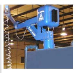
Gorbel's Easy Arm<sup>™</sup> has made loading and unloading two test stands in different work cells much easier for this pump manufacturer.
