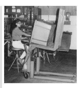
This company produces a wide variety of custom seals and gaskets for the automotive industry. After knitting, cutting, and performing, the preformed products are hand-picked from large tubs and placed in a press.
