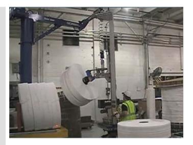
Before the Gorbel Easy Arm® was installed, it took two to three employees to move and stack the large 100 pound rolls of diaper material. This was an unsafe method and was the cause of increased labor costs and lower productivity.
