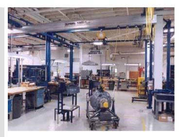
An aircraft maintenance re-manufacturing plant in Canada needed a safer, more productive process for disassembling and reassembling turbine engine reduction gear boxes without product damage.
