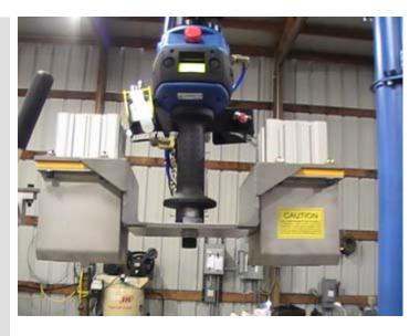
A manufacturer of log splitters is in need of a better way to handle hydraulic cylinders. The cylinders weight up to 70 lbs. They are manually lifted off a pallet, turned 180 degrees and set on conveyor. The cylinders are packed tightly on the pallet so that only the upper surface of them could be accessed.
