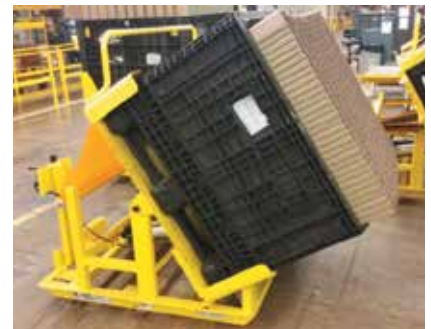
Kinetic Technologies’ tilt cart on riser is capable of a 60 degree tilt.
