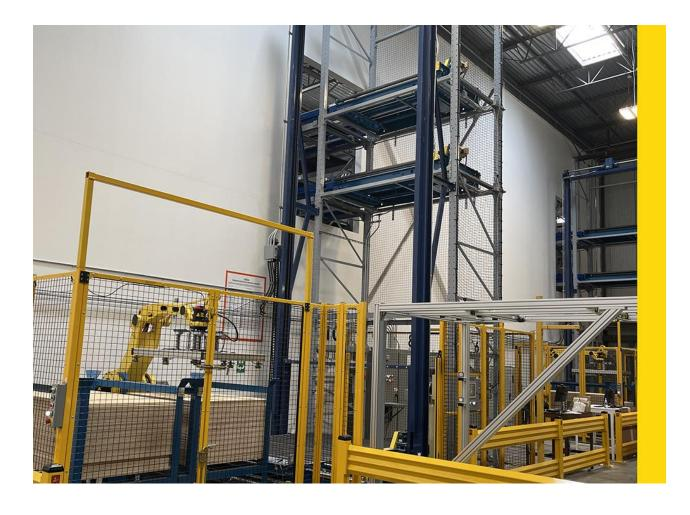
Our VRCs are working in tandem with the other automated systems and equipment to transfer the pallets to the storage areas in rapid time.
