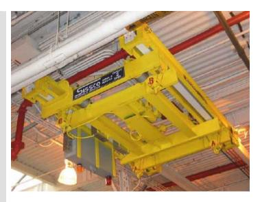
Two Pairs of independently controlled hooks with separate drive assemblies using variable frequency control for precise movement allows the A/C unit to be removed safely.
