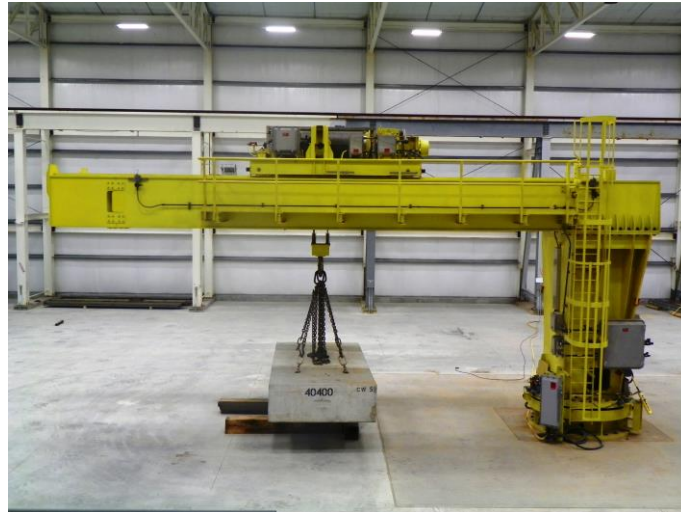
15 Ton Pedestal Base Mounted Jib Crane
