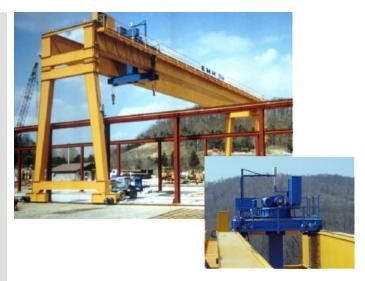
Outdoor Gantry with 120 foot span covers a 900 foot long loading area. Hoist with 360 degree rotation precisely handles loads to 30 tons.
