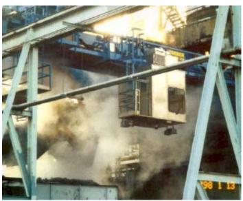
Maintenance cost was reduced to an estimated 10% of annual maintenance on the old cranes. PLC coordination of bucket hold and close hoists increased productivity.
