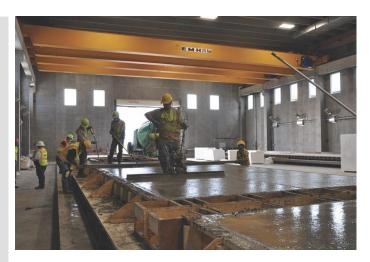
For Wells Concrete, four ZLX twin-girder twin-hook EMH Cranes were specified, each having a 25-ton capacity on 65-foot runways with 85-foot spans.
